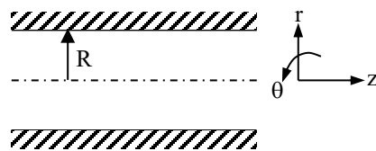
Figure 6.12 Geometry for a Poiseuille flow in a circular cross section pipe.
