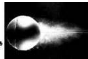
3. Turbulent separation behind a sphere
