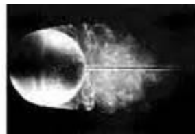
2. Laminar separation behind a sphere
